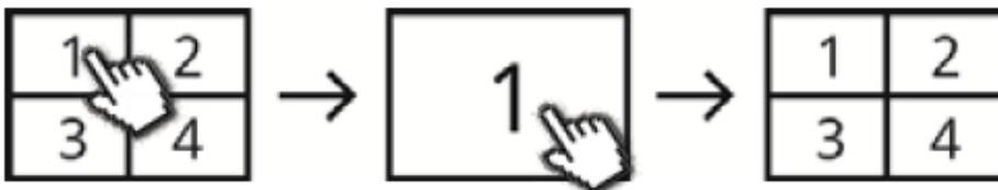
In the quad view, click on a channel using the left mouse button to display this as full-screen. Click on the full-screen again to change back to the quad view.
